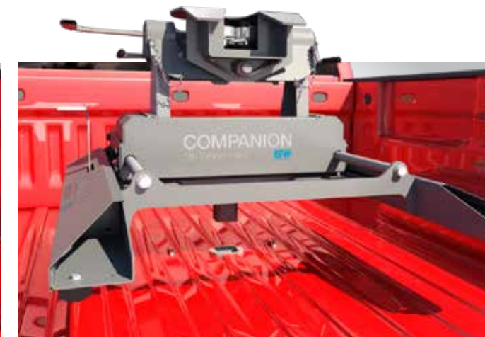
Companion Slider 5th Wheel RV Hitch Plug into the Turnoverball for extra turning clearance when towing a fifth wheel RV with a short bed truck.
